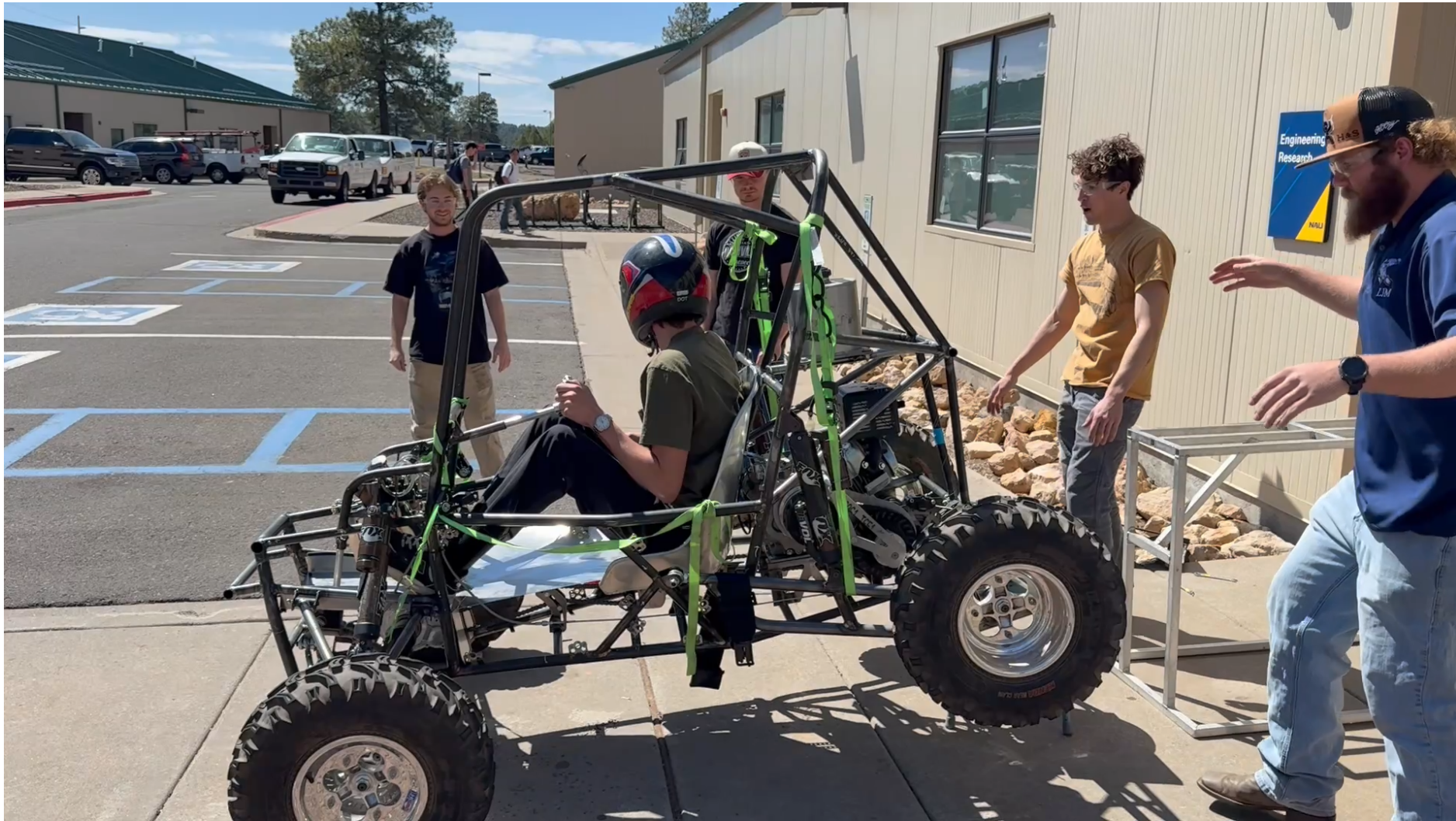
4WD Stool Test: Rear Tires Off the Ground to Show Front Drive Actuation
